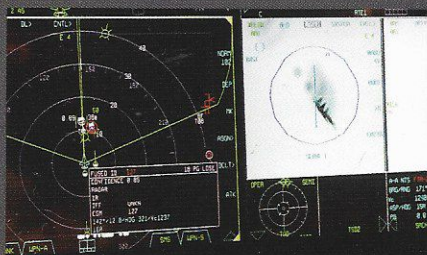
The main touch panel inside the F-35 cockpit. On the left is the Tactical Situation Display (TSD) that shows tactical information and a map centered on the aircraft. The right side shows a target captured by the Electro-Optical Targeting System (EOTS) displayed as a video image.
