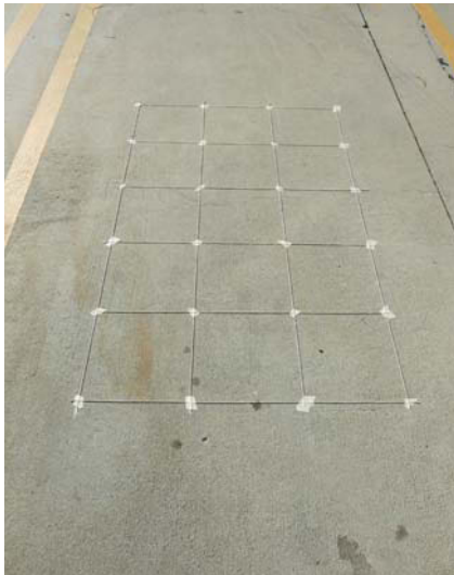
The string grid is placed on the working surface.
