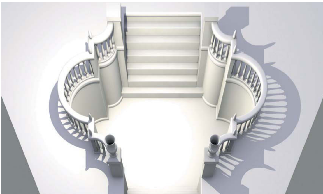
Step 2: For the second phase, digitally rendered components were created based on the black-and-white sketch to assess proper lighting and placement of the imagined architecture.
