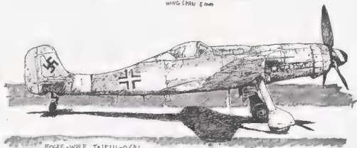
FOCKE-WULF TA 152H-0/1 TYPE, GERMAN HIGH-ALTITUDE FIGHTER POWER PLANT, ENGINE - JUNKERS JUMO 213B-1 CYLINDER LIQUID-COOLED ENGINE 1750 HP ARMAMENT, ONE 20-200 MK 108 CANNON TWO 20MM MK 101 51 CANNON MAXIMUM SPEED 322 m/h AT SEA LEVEL 465 m/h AT 25700 高度 60000 FT
