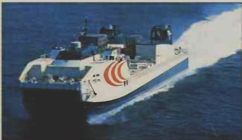
Hisho is a 70m (230ft) half-size model of the TSL-A. It is driven by two 16,000hp engines, linked to water jets.
