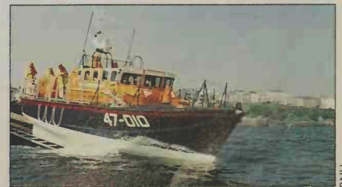
The side keels keep the lifeboat upright.
