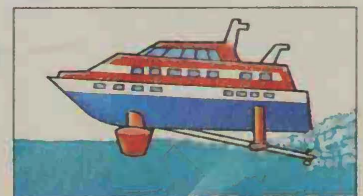
Going fast, the hull rides in the air. Only the foils stay underwater.
