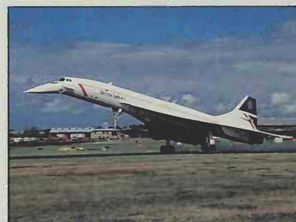
Concorde is powered by four Olympus 593 turbojet engines.
