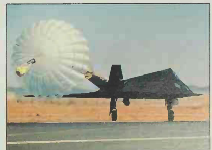
This F117A stealth fighter has used its brake parachute on landing.
