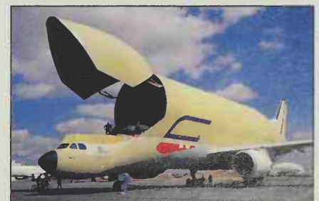
The A300-600ST's fuselage is over 7.2m (24ft) across.
