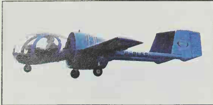
The Optica's cockpit gives a clear view all the way around. It is ideal for aerial observation and photography.
