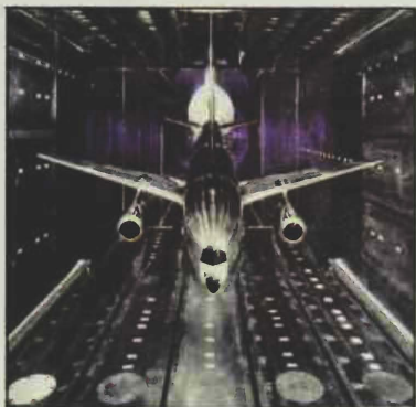
This airliner model is being tested in a high speed wind tunnel.
