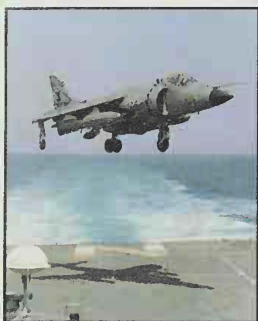
This Sea Harrier is landing vertically onto the deck of an aircraft carrier.
