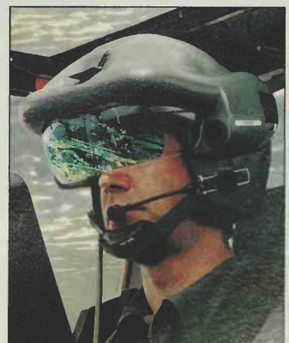
The projector in this helmet displays important information onto the pilot's helmet visor.
