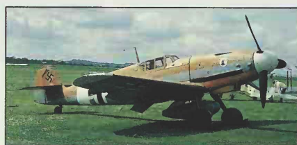
This German Bf109G has a stressed skin shell called a monocoque.
