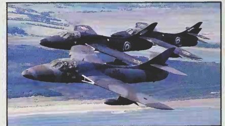
The Hawker Hunter's swept back wings helped it reach a top speed of over 1100km/h (690mph).
