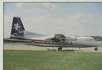
This Fokker F27 has two turboprops.
