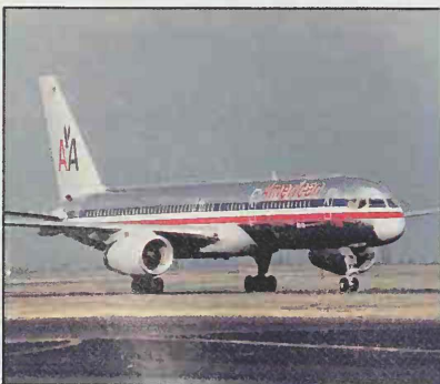
This Boeing 757 is powered by two RB211-535 engines.
