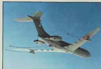
This VC10 tanker can supply planes with up to 86,000kg (190,000lb) of fuel through its three fuel probes.
